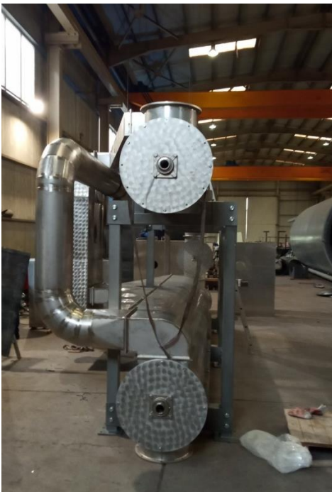
The dryer with the rack and the air inlet system
